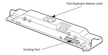
Figure 4-13 Port Replicator front panel
